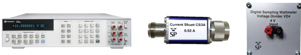
Figure 1. Components transferred in the intercomparison: digitiser, current shunt and RVD.
