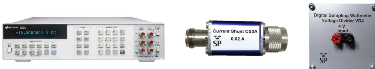
Fig. 11.1. Components transferred in the intercomparison: digitiser, current shunt and RVD.
