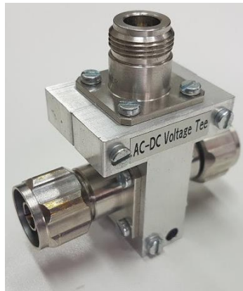
Fig. 9.9. AC-DC Voltage Tee used in difference comparator system.
