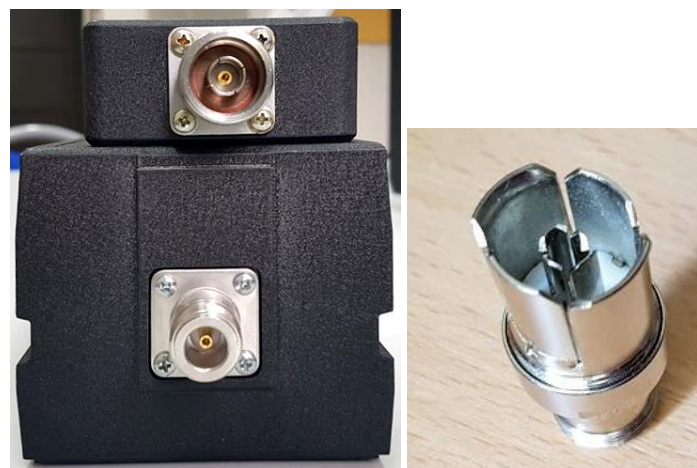
Fig. 9.7. Male (upper) and female (lower) N connector and GR874 hermaphroditic connector (right).
